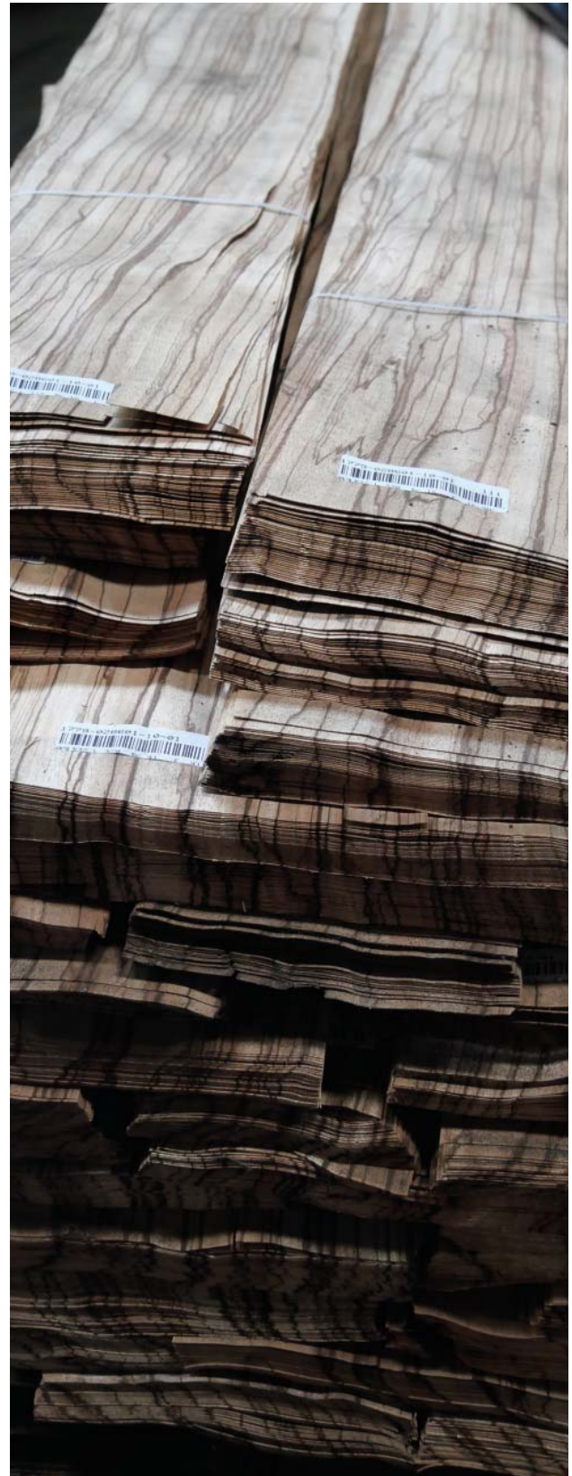
Fig. 19 | Bundled veneer stacks can be stored for years. Photo: IFN/Schlautmann
