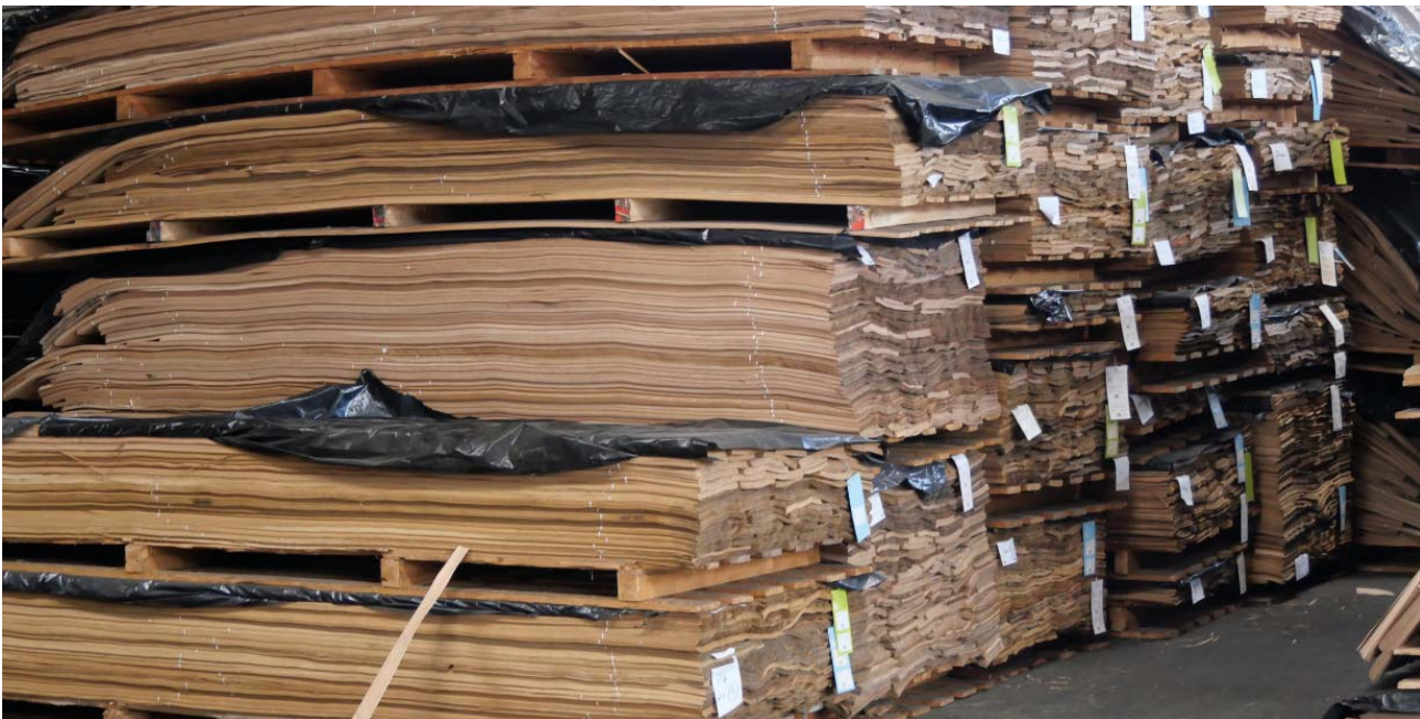
Fig. 22 | The storage of stacked veneer sheets is a natural UV protection.
