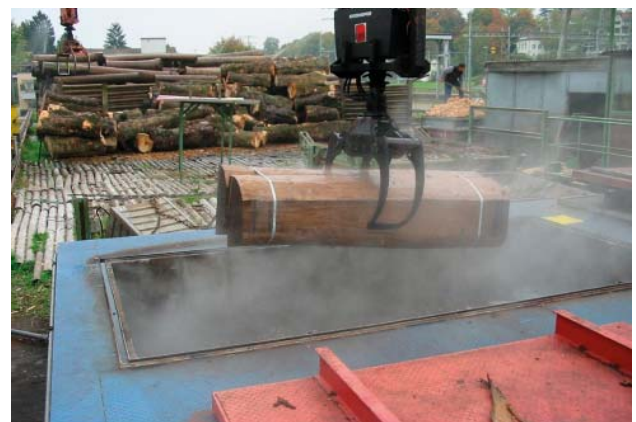
Fig. 7 | Steaming the veneer blocks Photo: Schorn & Groh GmbH
