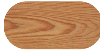
Fig. 26 | Crown figure in larch Source: Holzatlas
