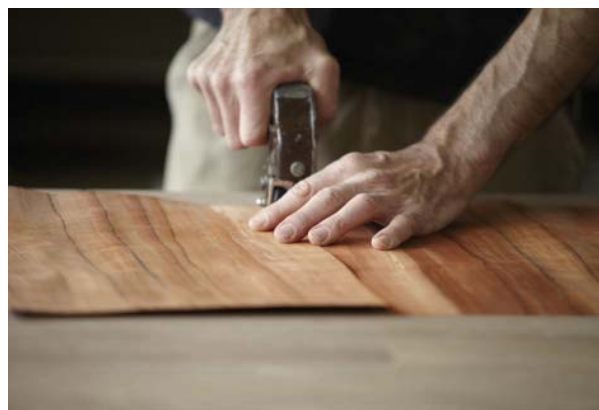
Fig. 5 | Veneer sheets are sewn together by hand or by machine. Photo: IFN
